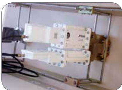
mounted on a Simulsat antenna feed
