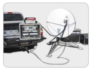
Our integrated and self-contained transportable rack contains all the electronic equipment necessary to uplink and monitor your program. Complete front access makes operating the system a user friendly experience.
