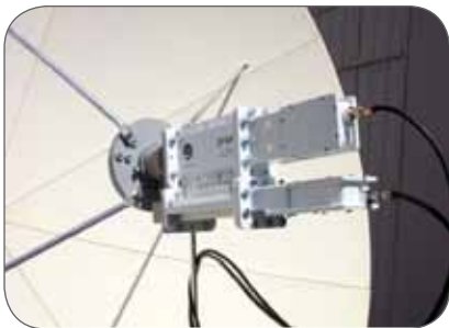
ZF100 mounted on a parabolic antenna feed
